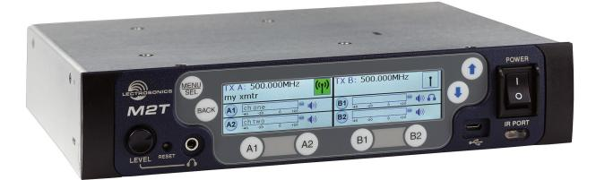
The M2T Digital Half-Rack Transmitter with analog and digital Dante™ network audio inputs presents an excellent sounding IEM system with a unique level of performance in a wireless in-ear monitor system. With ultra-low latency 24-bit audio, digital RF modulation and two stereo digital channels, the M2T provides a truly unique IEM product for demanding, professional applications.
