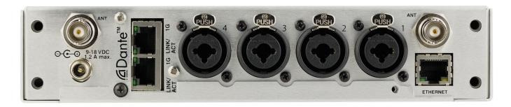
The M2T half-rack transmitter features transmission power of up to 50 mW for extended operating range. Locking XLR/TRS Combo connectors facilitate up to four channels of analog audio sources to be applied to the transmitter. A large, high resolution, backlit LCD and large membrane switches provide an intuitive interface.
