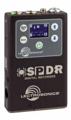
The SPDR is Lectrosonics' response to customer demand for a small, lightweight dual channel recorder for use on virtual reality sound captures or as a backup recorder for bag systems in the field. The SPDR will let you capture the full stereo audio of an extreme sport participant, in-car scenes or in situations where a wireless system cannot be used.
