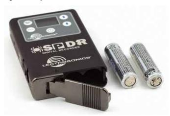
The SPDR has outstanding battery life (over 20 hours on AA lithiums) for long term recording capabilities when using only internal batteries. If external power is being used and is accidentally interrupted, a switchover to the internal batteries takes place automatically. The SPDR is compatible with the LM style transmitter belt clips. The wire belt clip (P/N 26526) is included and the hinged style belt clip (P/N BCHINGED) is available as an option.
