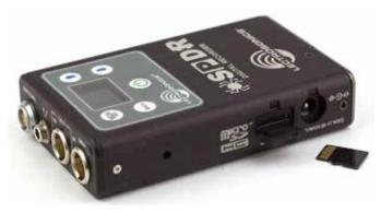
Attached cover protects the card slot from dust and moisture
